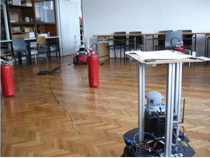
Fig. 1. Experimental setup of two laser range sensors calibration
