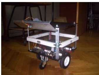
Fig. 12 Assembled mobile robot prototype
