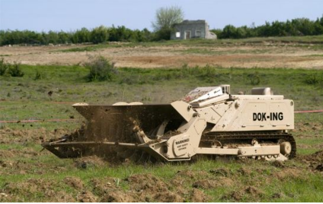
Fig. 1. The MV-4 mine clearance system. Courtesy of DOK-ING company www.dok-ing.hr .
