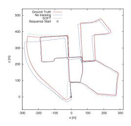
Fig. 6. Reconstructed path of the KITTI00 dataset
