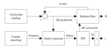
Fig. 3. Overview of the IMU fusion algorithm
