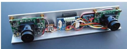
Fig. 4. Stereo camera with IMU
